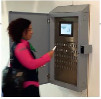
KeyConductor keeps a full audit trail of collected and returned keys, which can always be retrieved on the display, or which can be downloaded on a USB stick. Furthermore, the barcode version comes standard with a door and electronic lock.
